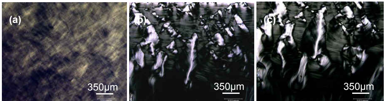
Figure 3.9 - Evaporation induced LC formation (a) Initial stage (b) Ordering at the edge (c) Growth of domains with time
